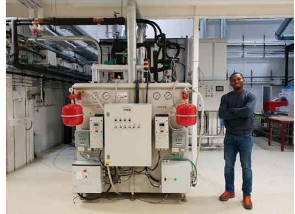
a) Process flow diagram of the butane-propane cascade laboratory prototype b) Picture of ventilated cabinet with the hydrocarbon high temperature heat pump
